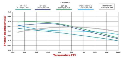
PM - ProMatrix Friction Coefficient and Temperature Values
